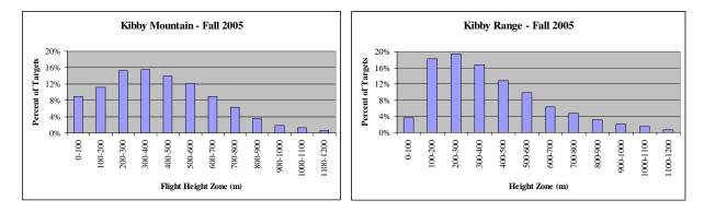
Figure 9 Target flight height distribution within 100 m (328 ft) height zones.
