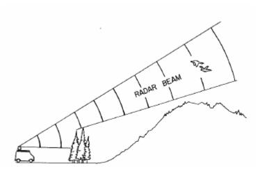
Figure 4 Example of how vegetation is used to screen out clutter-causing objects (taken from Sielman *et al.* 1981).
